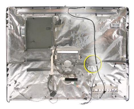
Remove any tape securing the camera cable to the rear housing. Lift the camera cable from the rear housing.
